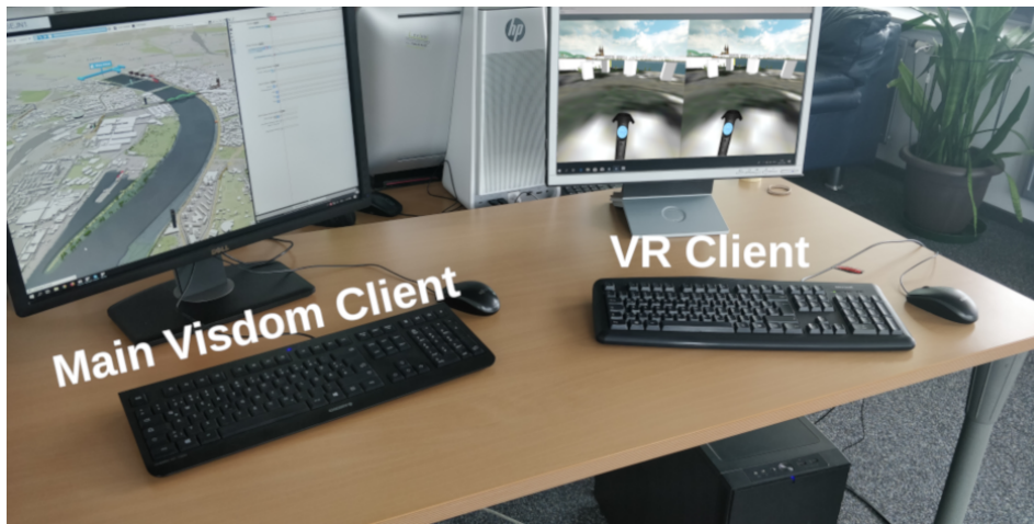
Figure 3.5: Basic Operator-Trainee setup. The operator-PC runs the Visdom Client and the other PC is responsible for running the VR application. Image has been taken by the author.
